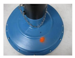
If the Aquasend Beacon is idle the magnet will cause it to begin telemetering. The Aquasend Beacon will announce that it is entering telemetering mode by a brief flash of its green LED indicators. If the Aquasend Beacon is in telemetering mode, the magnet will cause it to stop telemetering and become idle. The Aquasend Beacon will announce this transition by a brief flash of its red LED indicators.
