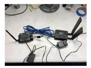
The Aquasend Beacon requires one of two types of Gateways: a DIGI ConnectPort X2 Gateway that is designed to plug onto the customer's local area network, or a DIGI ConnectPort X4 which is designed to connect to the public internet using cellular technology. Customers that require Verizon as their cellular provider will also get a DIGI WR11XT Transport modem device. This will be plugged into the DIGI ConnectPort X2.
