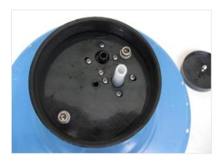
is accomplished by removing the cap and lifting off the sensor guard. This exposes the pumps, wiping mechanism, and sensor as pictured to the left.
